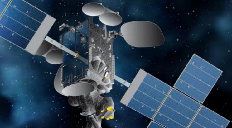
The Telestar 18 VANTAGE spacecraft is an advanced high-throughput satellite built by SSL of Palo Alto, California for Canadian company Telesat. In the coming days and weeks, it will use its own propulsion to establish a circular geostationary orbit where it will enhance broadcast capabilities through much of the developing markets of Asia with its Ku-band antennas and allow direct connectivity from Asia to the Americas with its broad C-band coverage.
